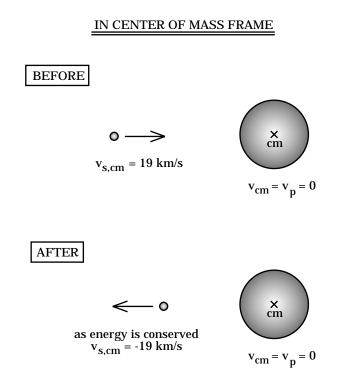
that the *satellite's incoming velocity* in that frame (i.e., in the center of mass frame) will be  $v_{s\ cm} = 7\ km/s + 12\ km/s = 19\ km/s$ .
