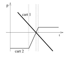
changing so the force is expected to be zero), increase suddenly to a constant positive value, then decrease back to zero. Note that the momentum vector changes direction when p = 0 (i.e., when the body stops). This has no special significance here. It means only that the force was applied long enough to stop the motion, then get the body moving back in the opposite direction. The *FORCE VERSUS TIME* graphs are shown to the right.
