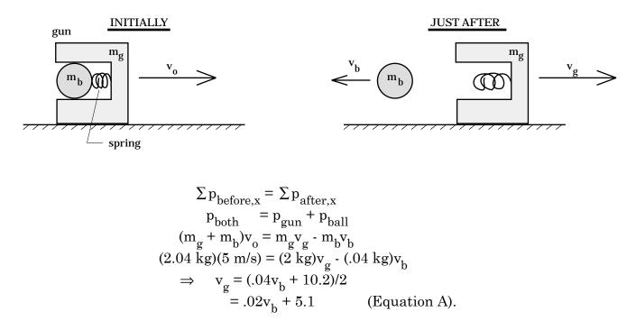
The spring is ideal so no energy is lost in the gun's firing. Using *conservation of energy* through the firing yields:
