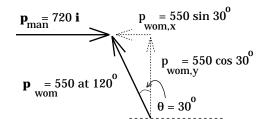
Remembering that the two individuals stick together (it is a *perfectly inelastic collision*), we can approach the problem by looking independently at what has happened to the system's momentum in the *x direction*, then *y direction*. Assuming the final velocity of the two is  $v_x$  in the *x direction* and  $v_y$  in the *y direction*, we can write:
