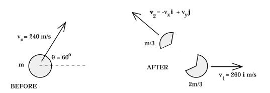
**a.)** Although there is gravity acting in the *y* direction, the explosion happens so quickly (i.e.,  $\Delta t$  is so small) that momentum will be "conserved through the explosion" in all directions. Writing out momentum considerations in both the *x* and *y* directions, and noting that the signs in  $v_x$  and  $v_y$  are unembedded, we can write:
